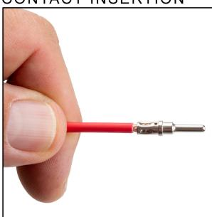
Grasp crimped contact approximately one inch behind the contact barrel.
