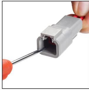
Step 6: To remove the contacts, gently pull wire backwards, while at the same time releasing the locking finger by moving it away from the contact with a screwdriver.
