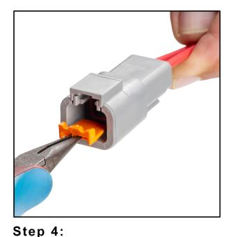
Once all contacts are in place, insert orange wedge. The orange wedge will snap into place.
