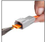
Step 5: Remove orange wedge using a flathead screwdriver to pry wedge straight out.
