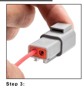
Push contact straight into connector grommet until a click is felt, A slight tug will confirm that it is properly locked in place.
