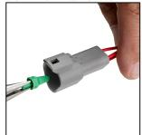
Step 5: Remove green wedge using needlenose pliers to pull wedge straight out.
