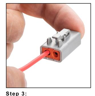
Push contact straight into connector grommet until a click is felt, A slight tug will confirm that it is properly locked in place.
