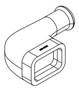
IF ADDITIONAL TAIL SEALING IS REQUIRED, A SHORT PIECE OF APPROPRIATELY SIZED ADHESIVE-LINED HEATSHRINK TUBING CAN BE USED. RECOMMENDED TUBING IS RAYCHEM TE ATUM-24/6-0-STK OR EQUIVALENT.
