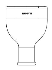
IF ADDITIONAL TAIL SEALING IS REQUIRED, A SHORT PIECE OF APPROPRIATELY SIZED ADHESIVE-LINED HEATSHRINK TUBING CAN BF USFD.
